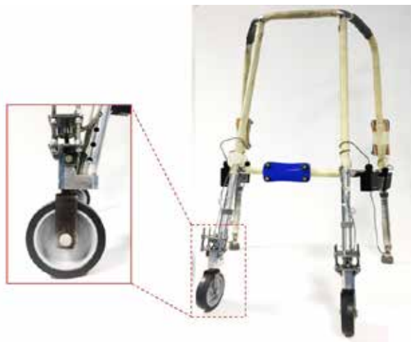
Figure 1. Example of a Smart Walker: front-wheeled walker with force-sensing load cells integrated into the front and rear legs.
